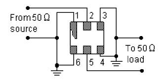
No impedance matching required for operation at 50  $\,$   $\Omega.$
